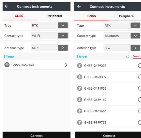
**Antenna Type:** Click **Antenna Type List**, select antenna type (Users can select antenna type of different products in different manufacturers). Users can handle specific item by clicking **Add**.
