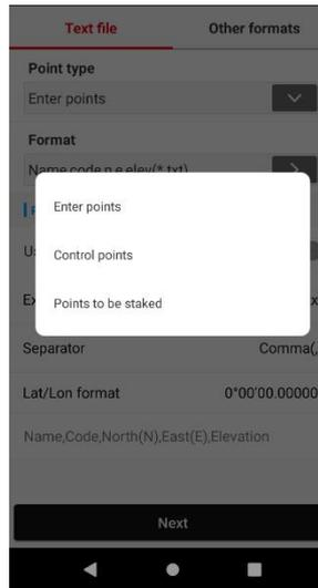
**Format:** user can select the target type from DAT, TXT, CSV, XLSX, and XLS. If the data contains table header, use header should be set by right slide menu.
