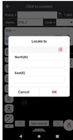
**Off set stakeout point:** Users could manually input coordinates, pick from the map, instant survey, or select from point library. After inputting distance and azimuth, click **Result** then input the **name** of the new point. Click **OK**.
