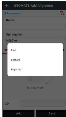
Input Length, Start offset, Start North, Start East and Azimuth if using specified azimuth. Click **OK** to finish adding.
