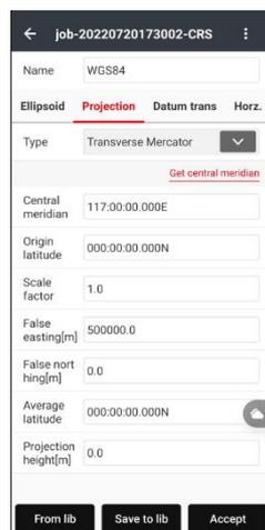
(3) **Datum Trans:** Represents the mathematical model for transformation between two coordinate systems. Datum transformation model includes none parameter, three parameters, seven parameters, seven parameters Bursa, and grid models. Users can input the local 7 parameters directly, no needing the site calibration any more.
