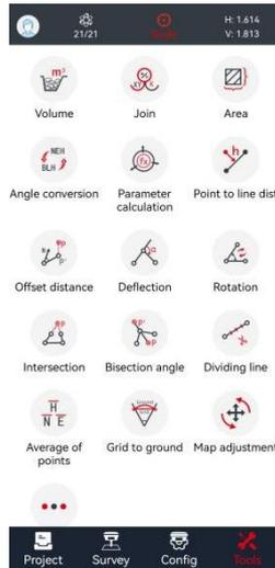
Tap **Grid to ground** in **Tools** interface. There are three methods to select grid coordinate: from Points, map selection and calculate directly. There needs two points for calculation, the first point coordinates are default as current base station coordinates. Grid scale factor, height scale and combined factor will be calculated after selecting second point coordinates. (Combined factor can also be inputted.)
