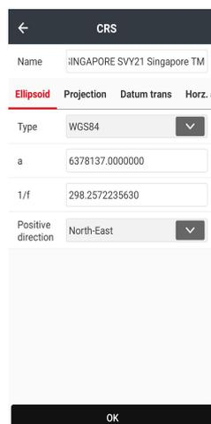
Users can view the parameters of ellipsoid, projection, datum transformation, Horz. adjustment and Vert. adjustment. Click **OK**, it'll return to **Coordinate System** interface, and then click **Select** to finish CRS configuration.
