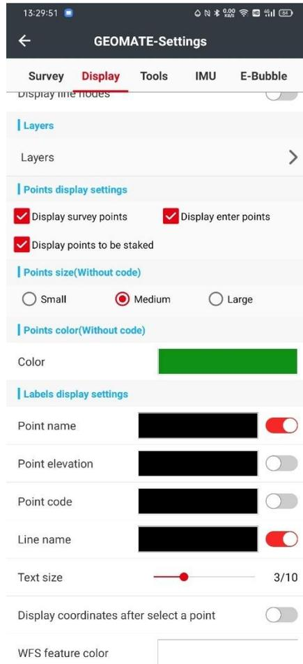
Different layers can be created, and you can choose to display different type of points and change the display of labels.
