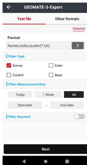
**Format:** Support DAT, TXT, CSV, XLSX, XLS. There are several available formats in common sequence that provides users to use and users can also set the format in **Customize** (users can customize the import contents while choosing the CSV, DAT and TXT format.)
