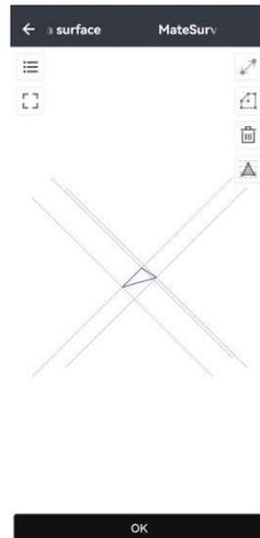
In this interface users can modify constraint line, boundary, and points of surface.
