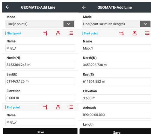
After setting the above values, click **Save**, a line can be created. Users can check the graph by clicking the rectangle button and inverse the direction by clicking the arrow button.
