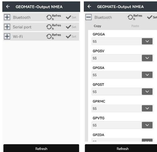
When users use receivers and set GPGGA output via serial port as 1Hz, please make sure that baud rate sets 9600.
