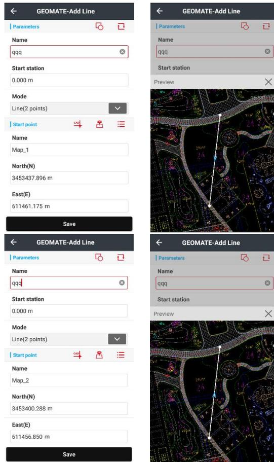
And there are 3 methods to select one point, including from CAD, from point survey and from point lists.
