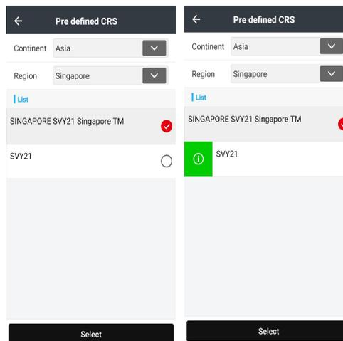
Click **Pre defined** to enter **Common Coordinate** interface, and then users are able to add a new coordinate system by clicking **Selecting**. Slide right and click the green button to check the coordinate system information.
