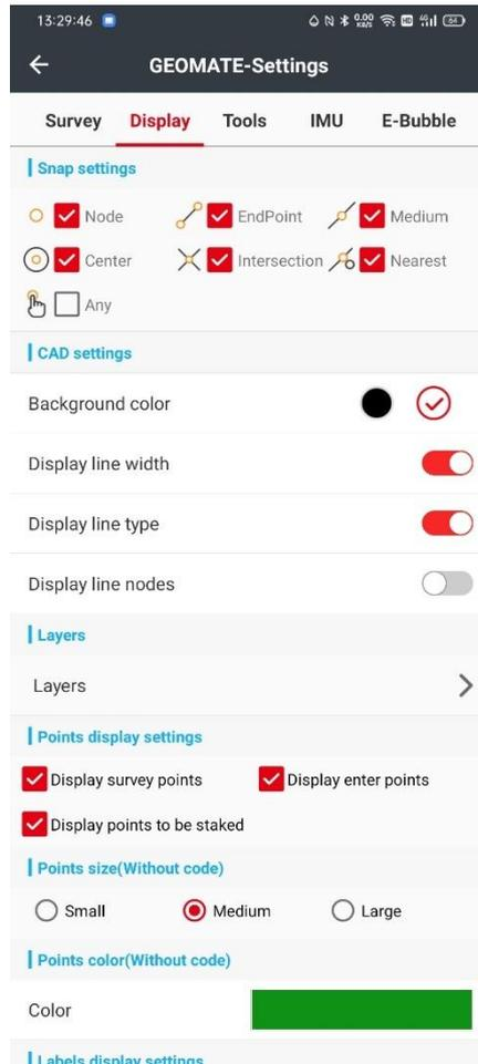
If you want the display of the line width and the line nodes, you can turn these buttons on. When opening a CAD map, you can change the unit and the coordinate system.
