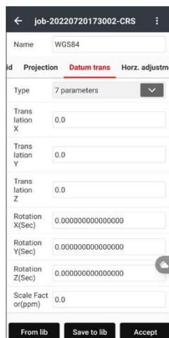
**Note:** When accuracy of known points is not high, 7 parameters transformation is not recommended.
