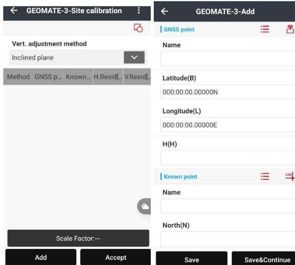
**Calculate:** Click **Calculate**. The software will prompt “Horz.adjust successfully”. After that click **OK**, it will make current calculated correction parameters apply in the coordinate system which can affect into the whole project.
