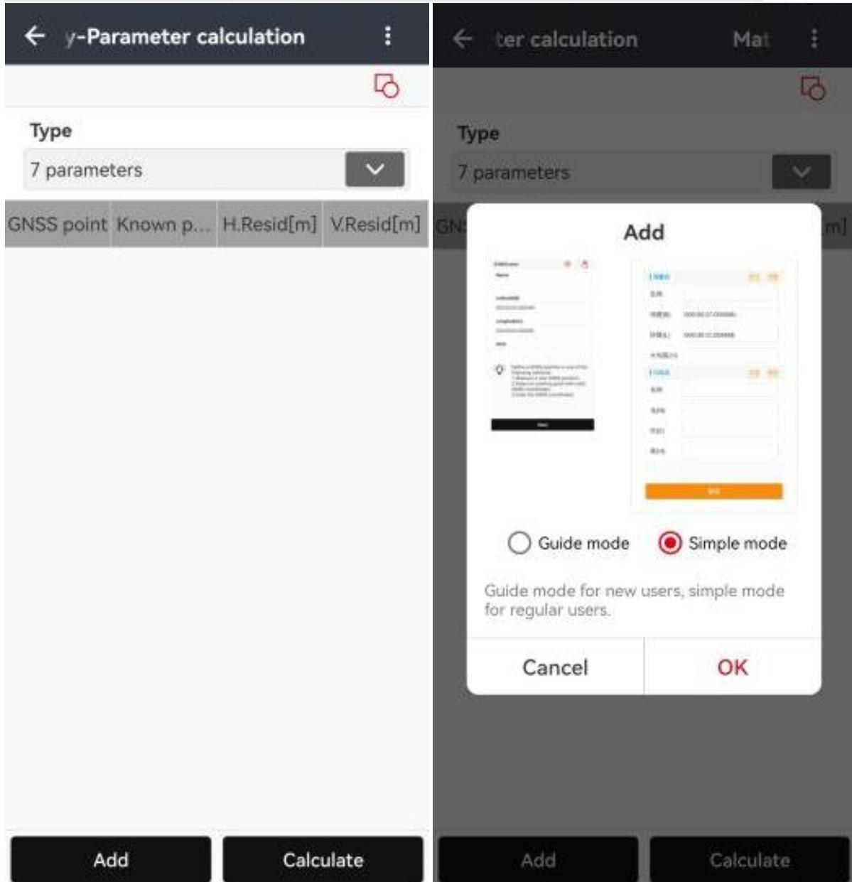
**Calculate:** Click to calculate. The results will be popped up automatically. Then click **OK** to apply the parameters to the current project.
