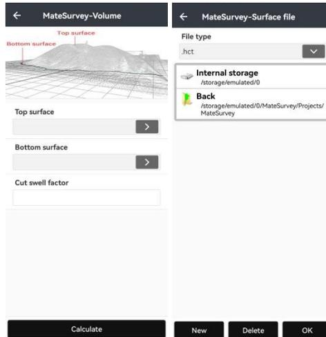
Users can choose surface file or create a new surface file by selecting points. Click **New** to create a new surface file, users can add a new point or select point in **Points**, then click **OK** to preview the surface.
