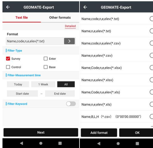
**Format:** Support DAT, TXT, CSV, XLSX, XLS. There are several available formats in common sequence that provides users to use and users can also set the format in **Customize** (users can customize the import contents while choosing the CSV, DAT and TXT format.)
