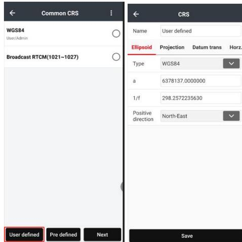
Set the right parameters according to the surveying area, and then click Save to finish CRS configuration.
