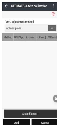
**Vert.adjustment Method:** Include Inclined plane, Constant adjustment, Surface fitting. Default plane fitting method is Inclined plane.
