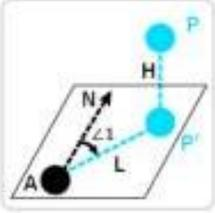
Known: point A, azimuth angle of AP, horizontal distance of AP and height difference.(N is north). Calculate: point P.
