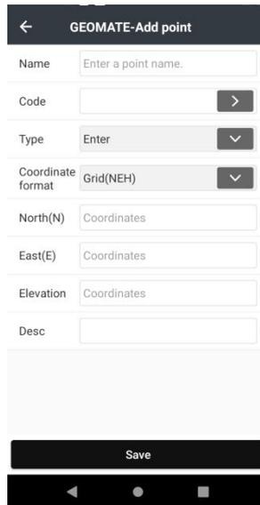
**Note:** When the point has reel number, it will prompt “Projection Error” after adding point, and users should add reel number in “False East” in **Projection** table of **CRS** interface.
