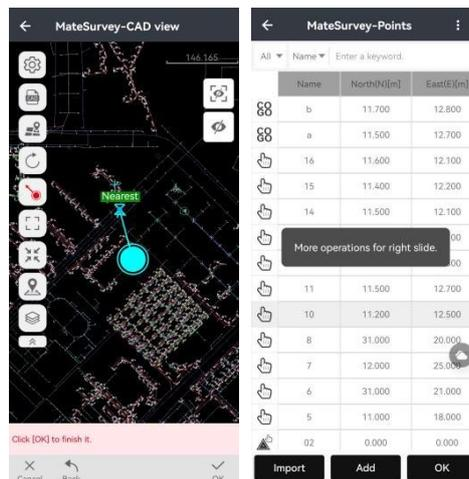
Click **Accept**, and then users will see transformed ground coordinates in point detail. There is no need to apply combined factor when it's 1, because default combined factor is 1 and users can view the ground coordinates in point detail directly. These ground coordinates can also be exported as TXT, DAT, or CSV format with customized content.
