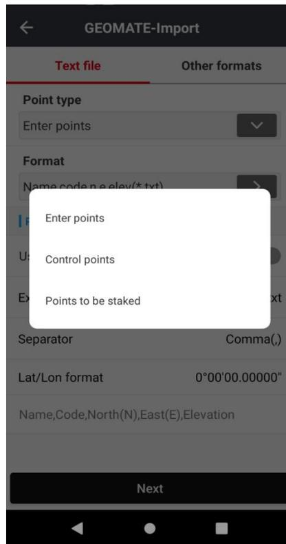
**Format:** user can select the target type from DAT, TXT, CSV, XLSX, and XLS. If the data contains table header, use header should be set by right slide menu.
