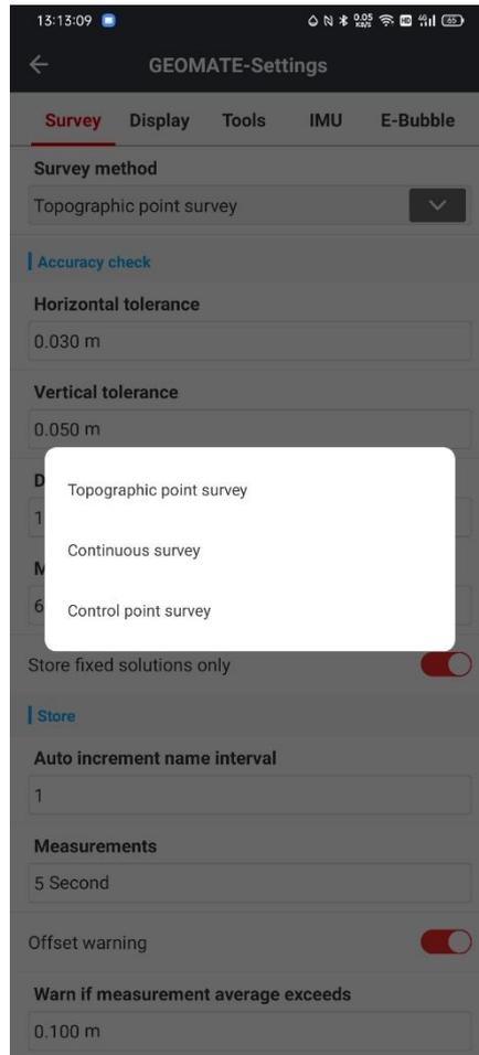
**Survey:** when doing the survey job, you can choose three different survey methods: Topographic point survey, Continuous survey and the Control point survey.
