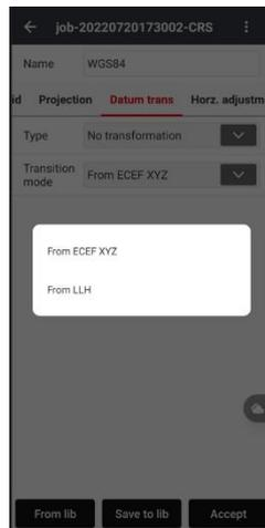
(b) **7 Parameters:** Requires at least three known points, and the points can be under the national coordinate system or the coordinate system that existing small rotation from the WGS84 coordinate system. Preferably three or more known points so that LandStar™ 8 can check the correctness. The mathematical model of this method is strict, and it is critical to the precision of the known points. This method is usually used in a wide-range work.
